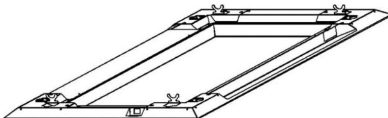
Line up the hooks with the receptacles on the IO1000, and gently push the fascia into position. The switch should be on the right hand side of the fire. The angle of the hooks can be adjusted if necessary to ensure a good fit.
