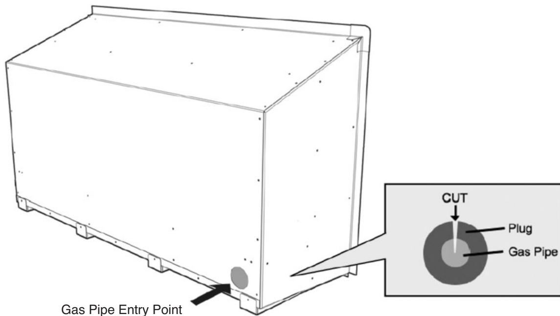
Any flexible pipe should be attached to the copper supply pipe and joint tested to ensure gas tightness, an isolating valve is recommended for this purpose.
