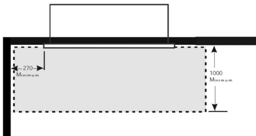
Minimum clearance distance between adjacent wall and fascia needs to be no less than 270mm.
