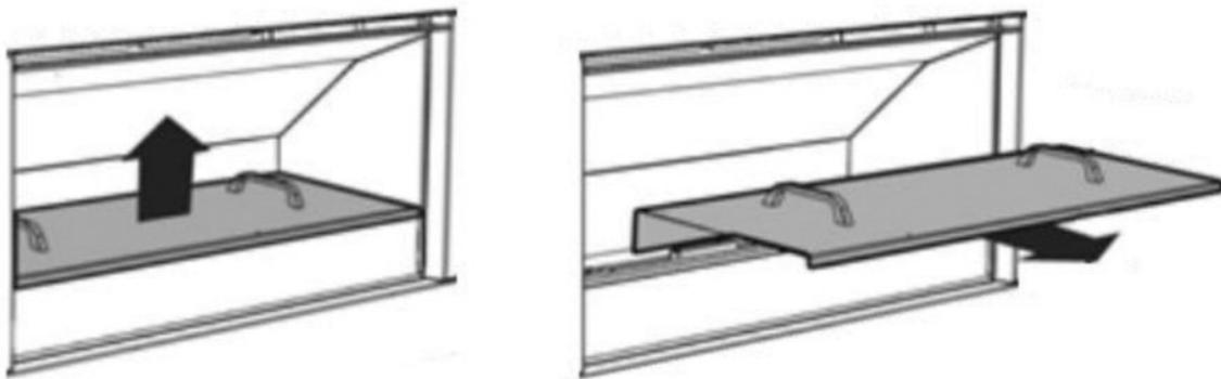
The cover **MUST NOT** be fitted while the fire is hot. A cooling period of 30 minutes must be observed before fitting.
